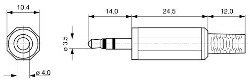
Cable diameter max. 4.0 mm
